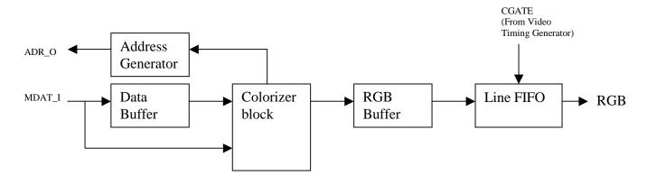
A block called the Color Processor, together with the Wishbone Master interface and the Line Fifo handles the pixel color generation. The internal structure of the Color Processor, including the Line Fifo and parts of the Wishbone Master interface is shown in the figure above.
