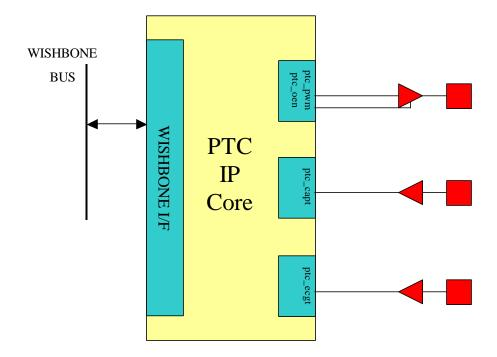
Figure 3. Core's Interfaces
