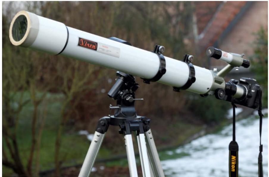
**A Vixen 80M refracting telescope with a Nikon D80 and a solar filter attached. A small astronomical telescope like this can be used with most DSLRs and is much cheaper than a super-telephoto lens.**
