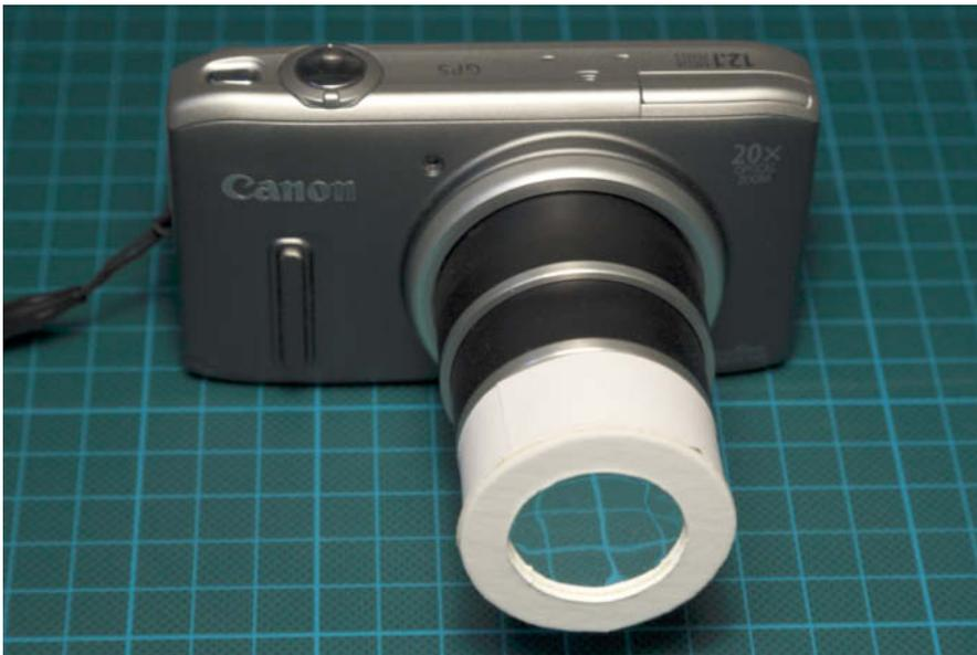
A Canon compact fitted with a home-made solar filter. The camera's 20x optical zoom is powerful enough to make large sunspots visible.
