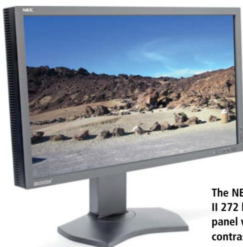
**The NEC SpectraView II 272 has an evenly lit panel with slightly less contrast than the competition**
