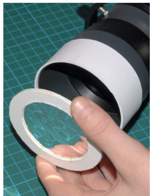
Fixing the filter to the tube
