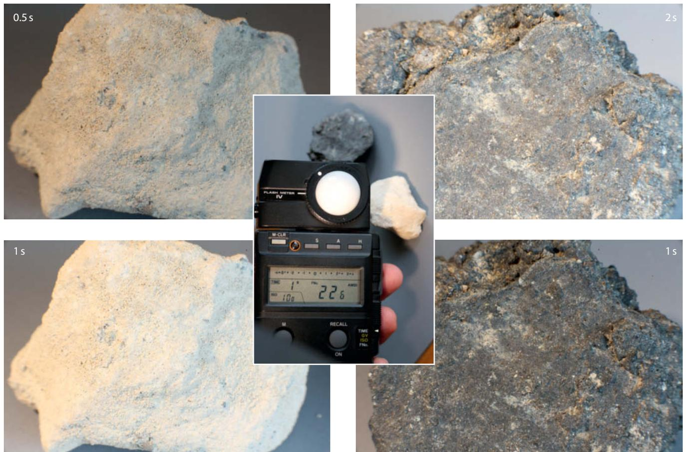
Using through-the-lens (TTL) metering to measure reflected light, our frame-filling test shot of a light-colored object turned out too dark (above left), while the darker object ended up too bright (above right). Metering the incident light produced more realistic-looking results (below left and right). The difference between the metered value of f22.6 and our setting of f22 compensated nicely for the loss of light produced by the long subject-to-focal-plane distance demanded by our close-up.
