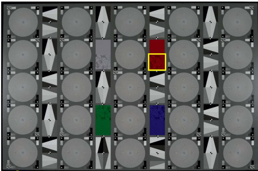
The 25 Siemens stars in our lab test scene cover most of the image area and enable us to produce reliable resolution measurements all the way into the corners of the frame. The abstract patterns outlined in the yellow border are great for revealing weaknesses in the reproduction of detail contrast.
