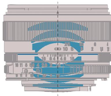
The simple Planar construction (left) used in many standard lenses compared with the more complex Distagon geometry (right) used in the high-end Zeiss Otus 55mm f/1.4 lens.
