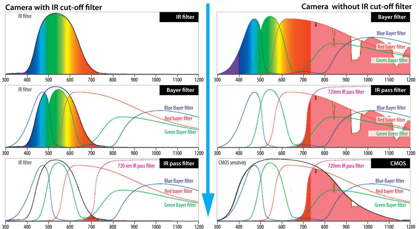
Each filter layer cuts off some of the light entering the lens. If an additional IR pass filter (in this case with a 720nm threshold wavelength) cuts out invisible light too, virtually no light will reach the sensor in a conventional unmodified camera (left). In a camera without a built-in IR filter, the sensitivity to IR light is determined by the limits of the sensor's own sensitivity (right). These diagrams are based on typical curves.
