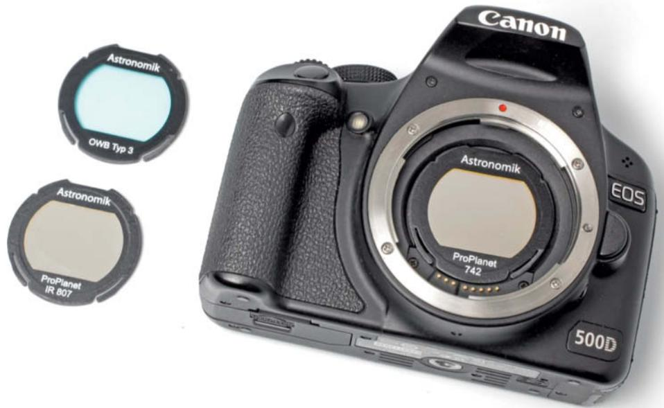
The clip-in filters from <http://www.astronomik.com/en/> are available to fit a wide range of APS-C and full-frame Canon bodies but cannot be used with EF-S lenses, which protrude too far back into the camera body
