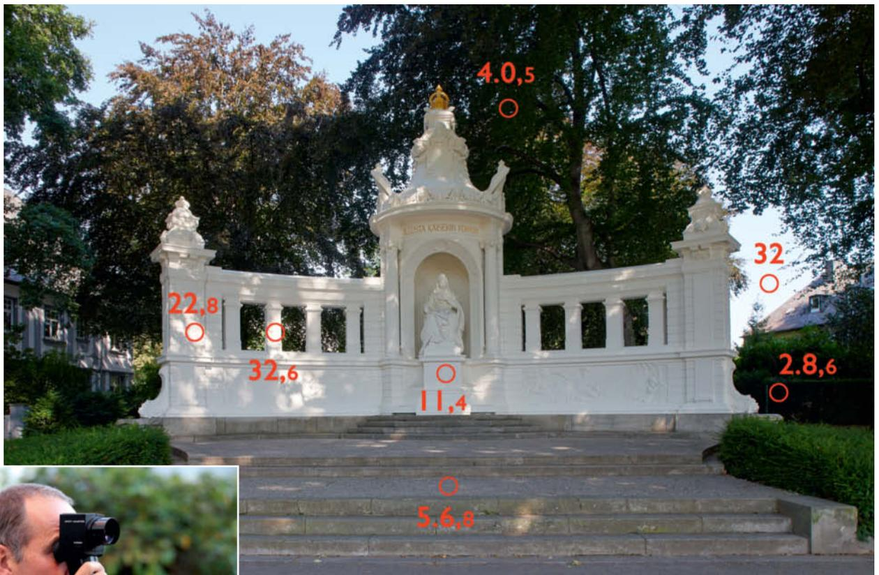
A handheld spot meter can be used to precisely determine the distribution of tonal values within a subject. The Gossen Spot-Master shown here (now superseded by the Mavo-Spot model) is often used to meter exposure for traditional black-and-white photography according to the tenets of the zone system. The illustration shows the spot meter readings for various zones in the subject.
