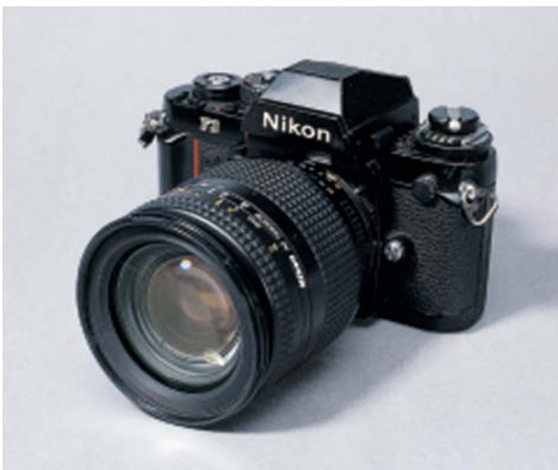
**Kodak based its first pro-grade DSLR (in 1991) on a tried-and-trusted workhorse – the Nikon F3, which was still the epitome of the indestructible professional press camera despite its lack of autofocus and its old-school technology**
