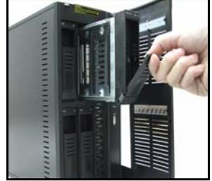
3 Place the disk tray on a flat surface with the panel facing up. Place a hard disk with the screw holes facing up on the same surface and slide it into the disk tray. Secure it with the screws as shown.
