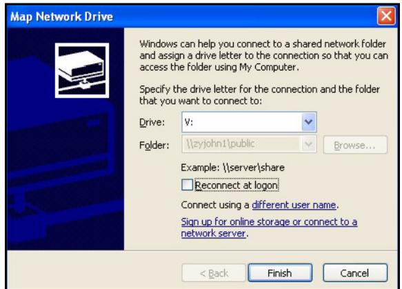
Alternatively (from another computer that does not have NDU installed for example), open Windows Explorer and type two back slashes followed by the NSA system name or IP address.
