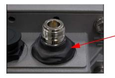
4 Connect the supplied antennas to the top antenna connectors (these are for the ZyAIR's WLAN 1 adapter). When facing the rear of the ZyAIR, the left antenna (main antenna) transmits and receives, the right antenna (receive diversity antenna) only receives.
