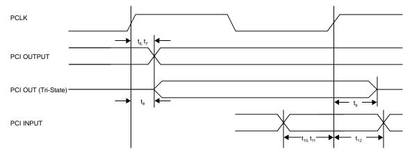
Figure 17 PCI Signal Timing<sup>1</sup>
