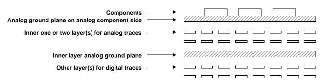
Figure 28 Analog Components on One Side of the PCB
