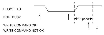
Figure 14 Command Transfer Timing
