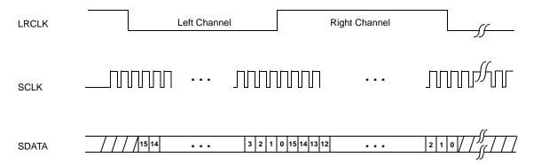
Figure 24 I2S Digital Input Format
