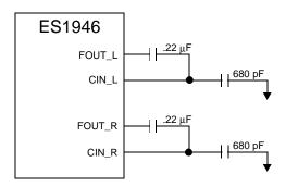
Figure 13 Switched-Capacitor Filter Pin Diagram
