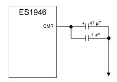
Figure 12 Reference Generator Pin Diagram
