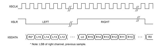
Figure 19 I2S Digital Input Format
