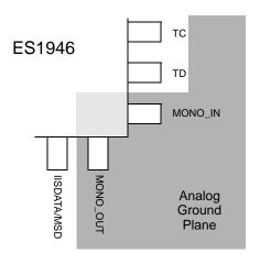
Figure 11 Analog Ground Plane Diagram
