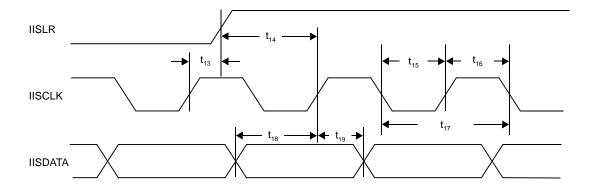
Figure 18 Serial Input Timing for I2S Interface
