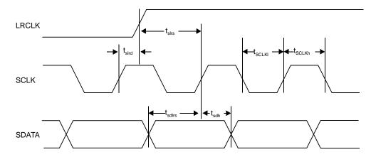
Figure 23 Audio Interface Timing
