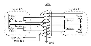
Figure 7 Dual Joystick/MIDI Connector
