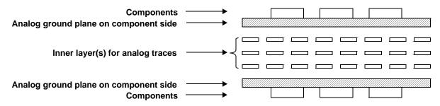
Figure 29 Analog Components on Both Sides of the PCB
