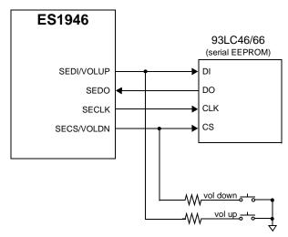
Figure 10 Serial EEPROM - Typical Application
