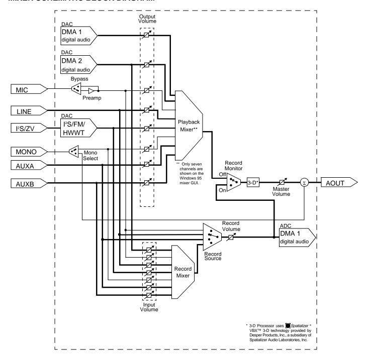
Figure 4 ES1946 Mixer Schematic Block Diagram
